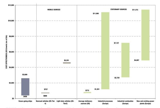
FIGURE 18. Comparing the Cost Effectiveness of SO<sub>x</sub> Control Options for Various Source Categories (Entec 2005c, US EPA 1999, 2004, 2005)
