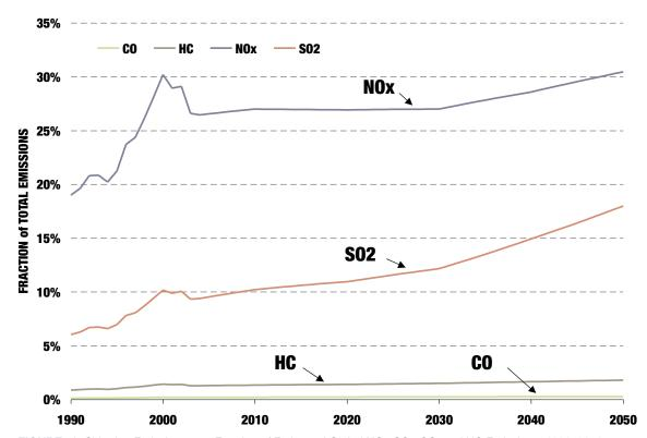
FIGURE 12. Shipping Emissions as a Fraction of Estimated Global NO<sub>x</sub>, SO<sub>2</sub>, CO, and HC Emissions: 1990–2050
