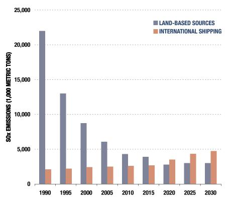
FIGURE 7. Projected SO<sub>x</sub> Emissions in Europe from Land-based and International Shipping Sources (EC 2005)
