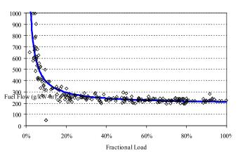
FIGURE A-5. Specific Fuel Consumption for Marine
