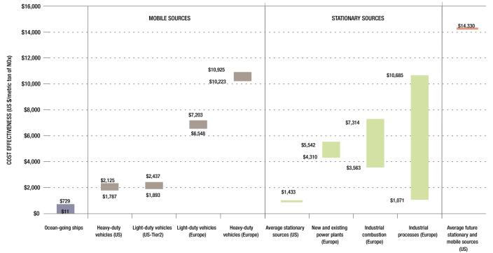
FIGURE ES-4. Comparing the Cost-Effectiveness of NO<sub>x</sub> Control Options for Various Source Categories (Entec 2005b, US EPA 1999, 2000, 2005)
