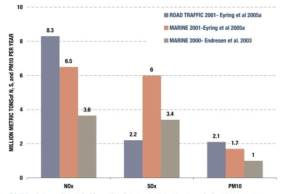
**FIGURE 6.** Estimated Global NO<sub>x</sub>, SO<sub>x</sub>, and PM<sub>10</sub> Emissions for Marine Vessels and On-Road Vehicles in 2001 (Eyring et al. 2005a, Endresen et al. 2003)
