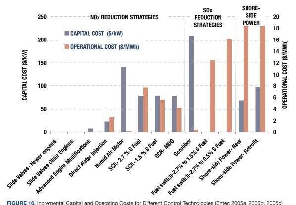
FIGURE 16. Incremental Capital and Operating Costs for Different Control Technologies (Entec 2005a, 2005b, 2005c)
