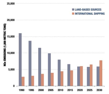
FIGURE 8. Projected NO<sub>x</sub> Emissions in Europe from Land-based and International Shipping Sources (EC 2005)
