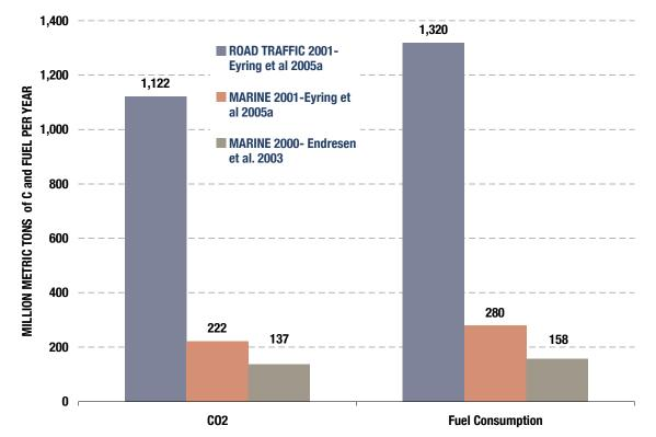
**FIGURE 5.** Estimated Global CO<sub>2</sub> Emissions and Fuel Consumption for Marine Vessels and On-Road Vehicles in 2001 (Eyring et al. 2005a, Endresen et al. 2003)
