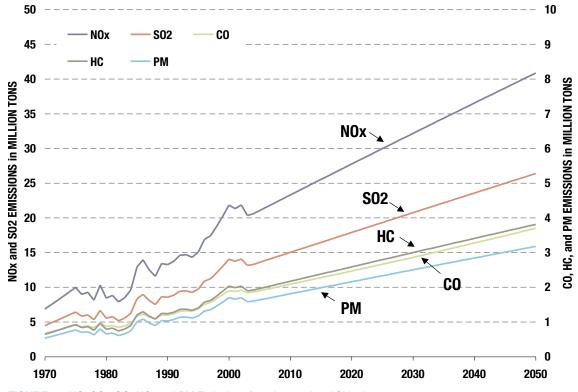
FIGURE 11. NO<sub>x</sub> SO<sub>2</sub>, CO, HC, and PM Emissions from International Shipping: 1970–2050
