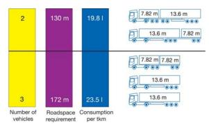
Practical test results with EMS vehicle combinations have demonstrated a reduction of 32% in the number of trips, a 23% reduction of transport costs, a 15% reduction of fuel consumption, a 15% reduction of  $CO_2$ emissions, a better utilisation of available drivers and a 5% increase in road longevity.
