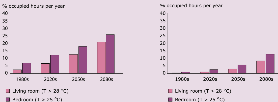
Figure 2.24 Discomfort temperature as built (left) and as adapted (right)
