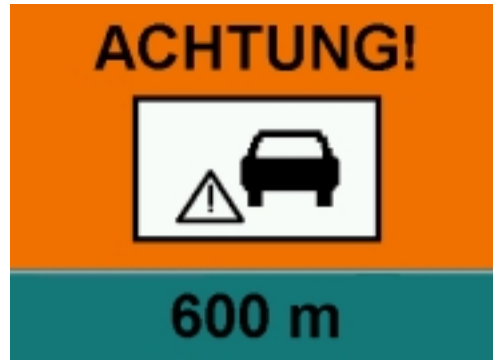
Figure 9: IVHW-Display for the hazard type "Breakdown"
