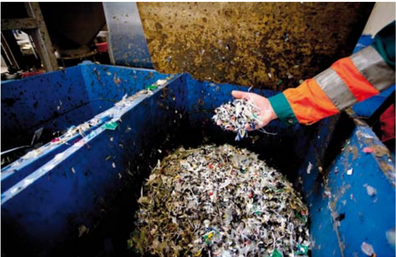
Residual plastic material from packaging accumulated during the production of biogas from waste food
