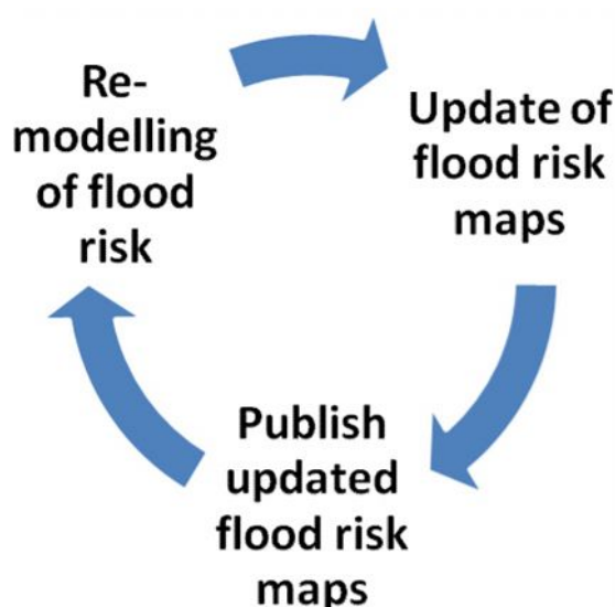
Figure 9.5: The flood mapping cycle
