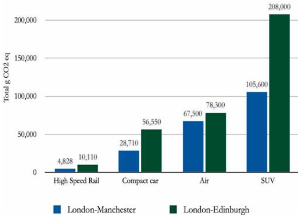
Figure 2.4: Direct emissions from relevant transport modes for middle London-Manchester) and long (London-Edinburgh) distance domestic journey scenarios.
