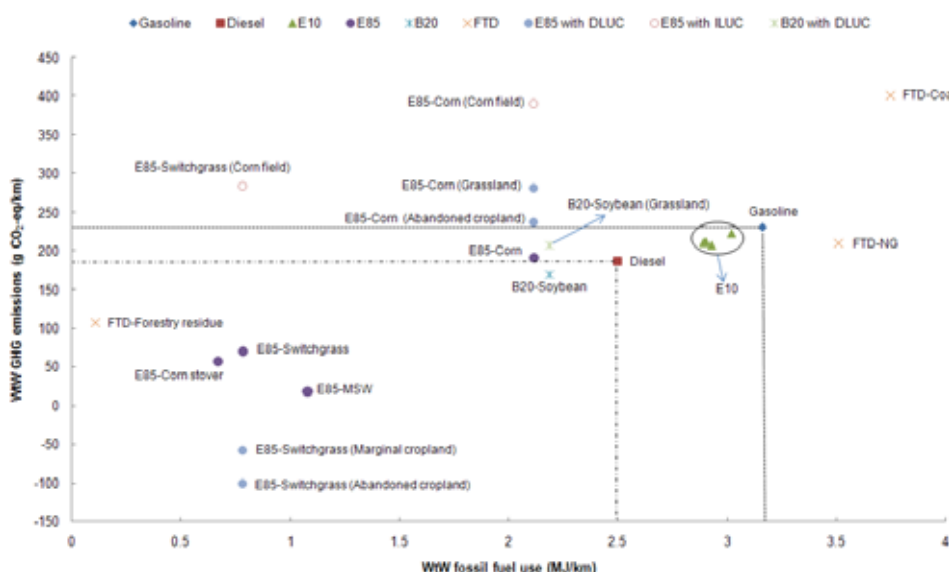
Figure 2.2: Life cycle fossil fuel use and GHG emissions 'per vehicle kilometre travelled' for biofuels and synthetic fuels in the US [202]
