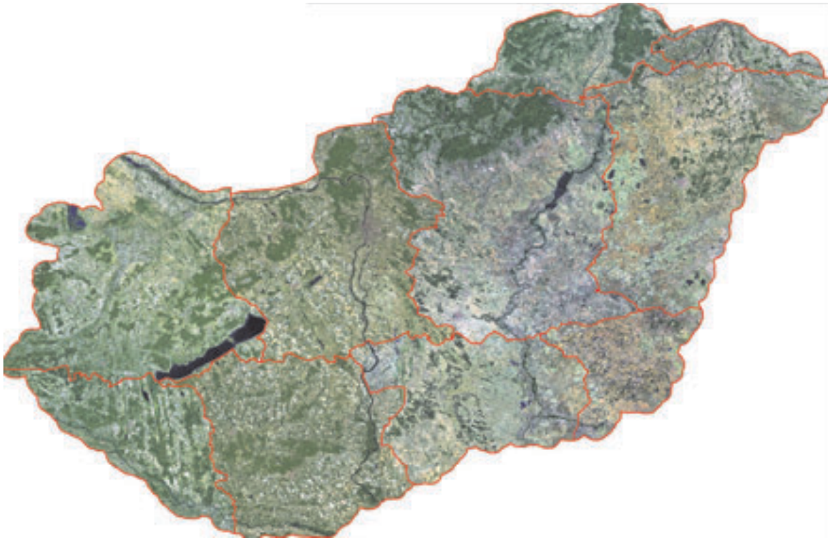
Figure 39- Overview of country mosaic for Hungary (band combination 7-5-3), overlaid with mosaicking lines, with 5km buffer along country boundary.
