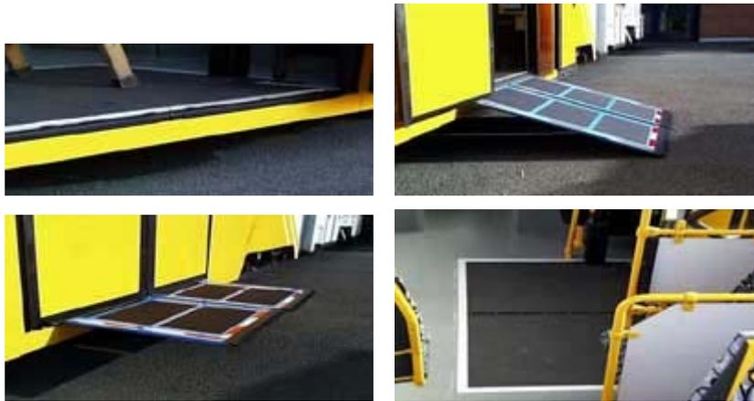
**FIGURE 43 : SEQUENCE DE DEPLOIEMENT DE LA RAMPE D'ACCES D'IBEG**
