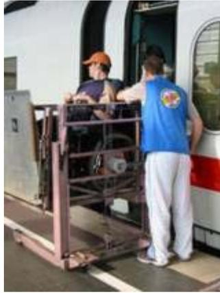
**FIGURE 15 : SYSTEME MOBILE POUR L'EMBARQUEMENT A BORD D'UN ICE**
