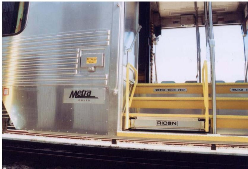
**FIGURE 4 : PLATE-FORME ELEVATRICE RICON EN POSITION REPLIEE**
