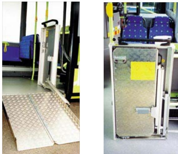
**FIGURE 30 : RAMPE D'ACCES DART POUR AUTOBUS**
