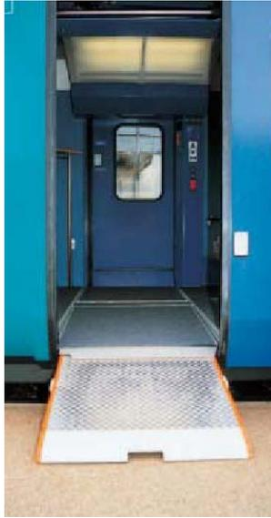
**FIGURE 40 : APPLICATION FERROVIAIRE D'UNE RAMPE D'ACCES DE LA DIVISION IFE**
