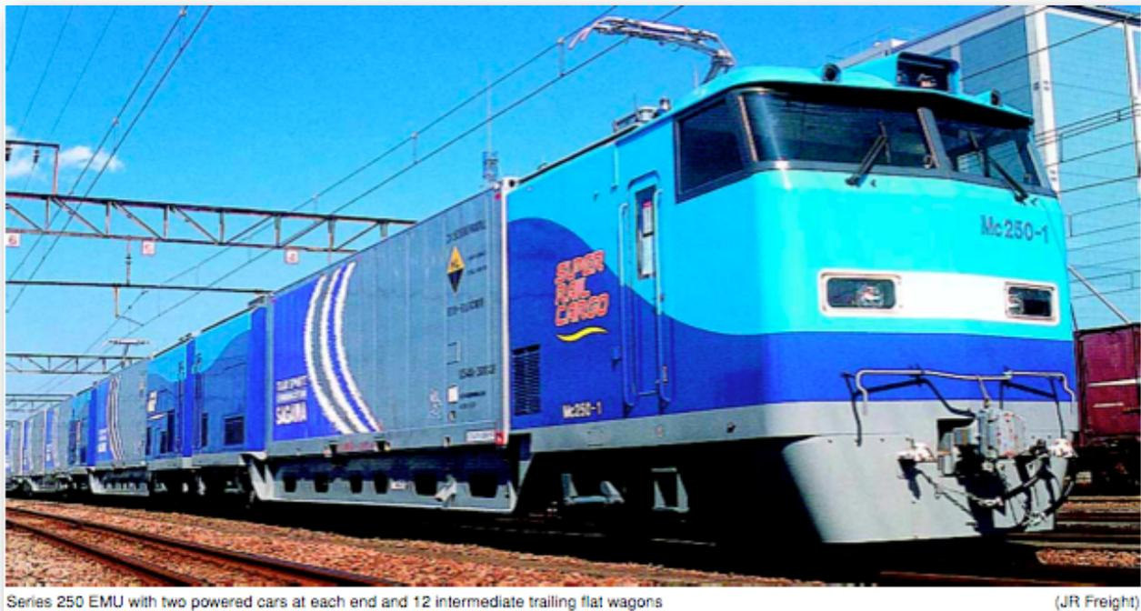
Series 250 EMU with two powered cars at each end and 12 intermediate trailing flat wagons
