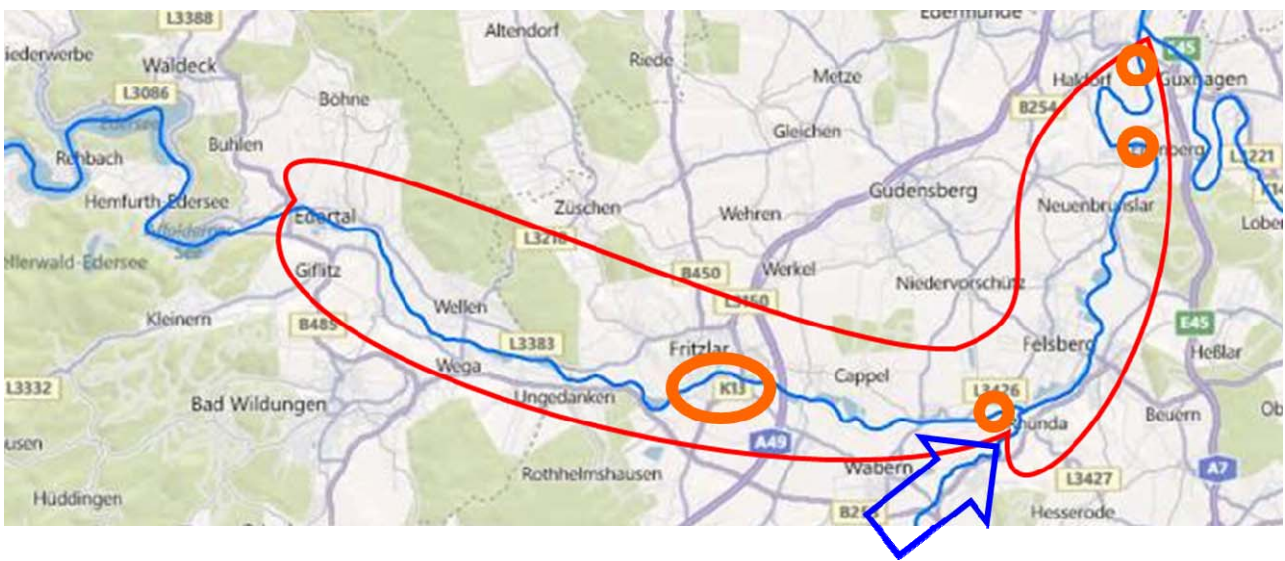
Figure 27: Map of the total 44 km long reach of the Lower Eder River including water releases and the confluence of Schwalm River investigated for effects of climate change on hydromorphology in comparison to human impact by stream training
